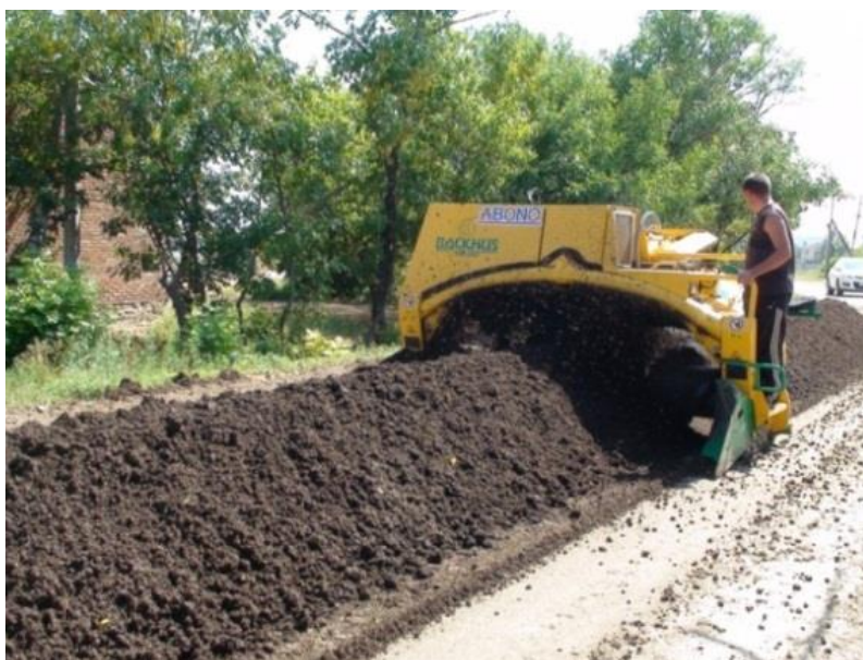
Figure 6 – Overview of COF production space using the accelerated composting technology at an open space
